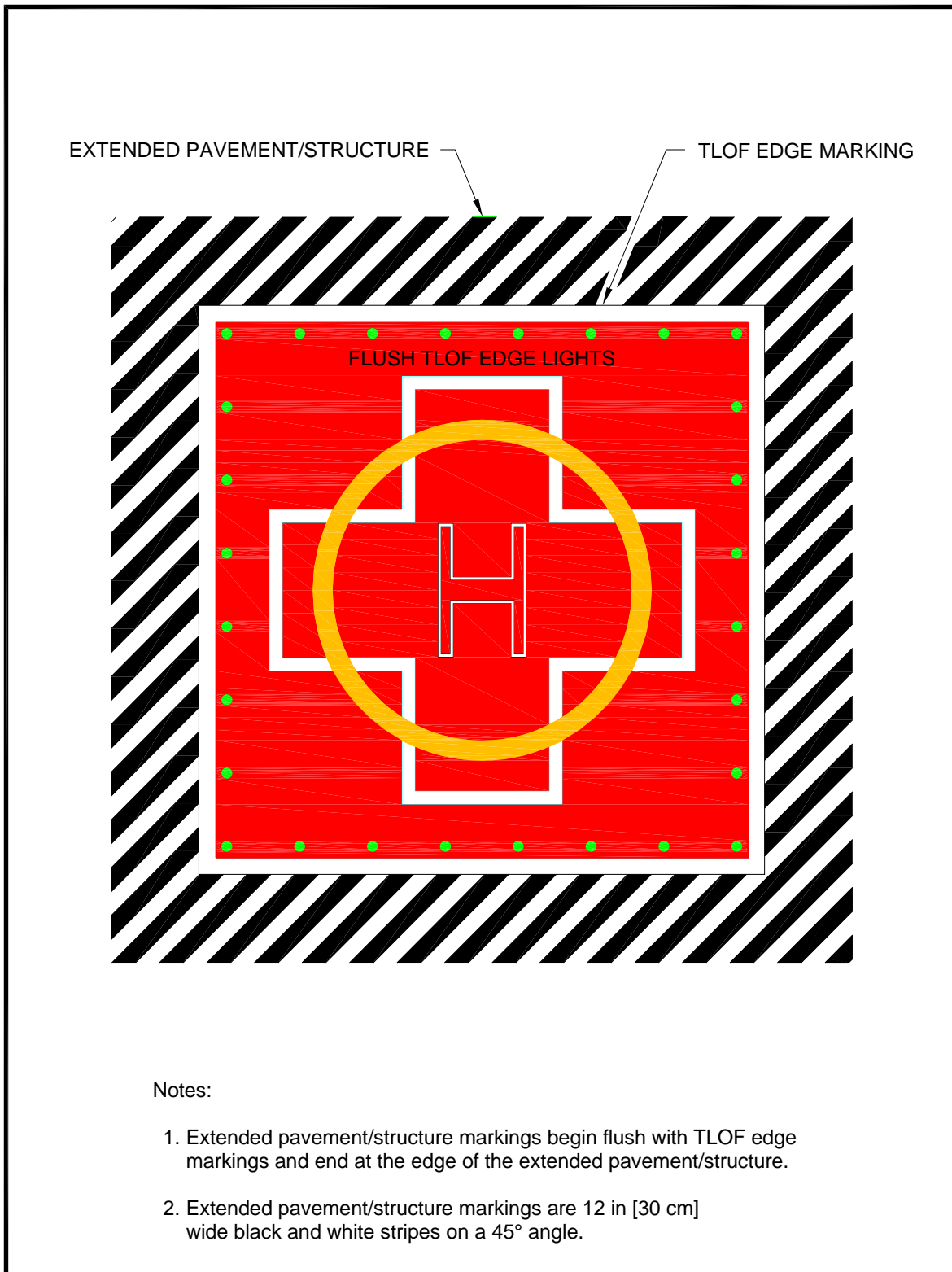
Figure 4–26. Extended Pavement or Structure Marking: Hospital
